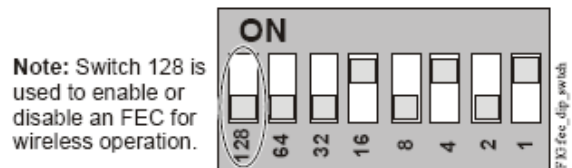
Figure 9: Device Address Switches Set to 21
